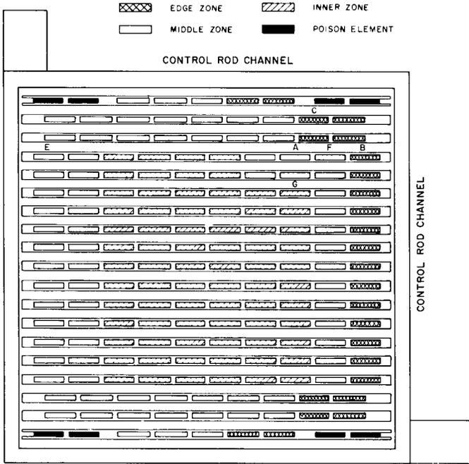
FIGURE 1.3. Shippingport Core 2 Seed 1, New Zoning of Seed to Optimize Power Distributions, Taking into Account Intrawater Flux Gradients.
