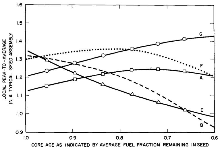
FIGURE 1.5. Shippingport Core 2 Seed 1, Peaking Factor Lifetime Variation as Calculated for New Zoning (A, B, E, F, and G represent various points within the fuel assembly shown in Fig. 1.3).
