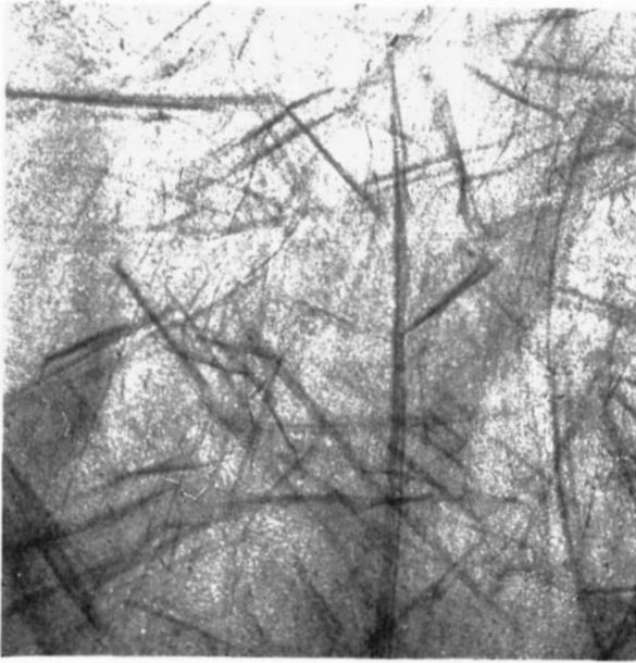
Fig. 9(a). Polycrystalline beryllium as cast. Iron radiation.
