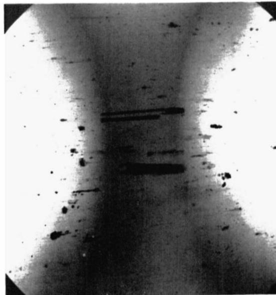
Fig. 3. Extruded beryllium with heavy included material. Copper radiation. Magnification  $\times 1\frac{1}{2}$  to  $\times 10$
