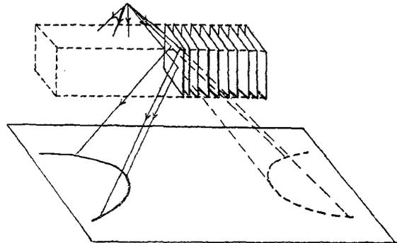
Fig. 6. Diagrammatic representation of the formation of deficiency and reflexion conics
