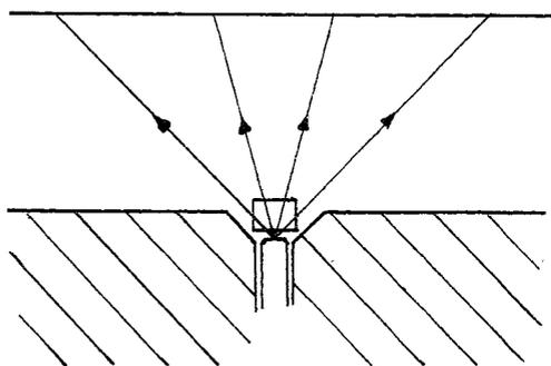
Fig. 1. Experimental arrangement of the X-ray microscope
