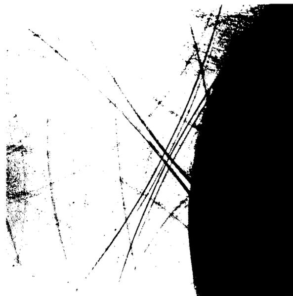
Fig. 8. Impure end of a zone-refined crystal of beryllium. Copper radiation. Magnification  $\times 20$
