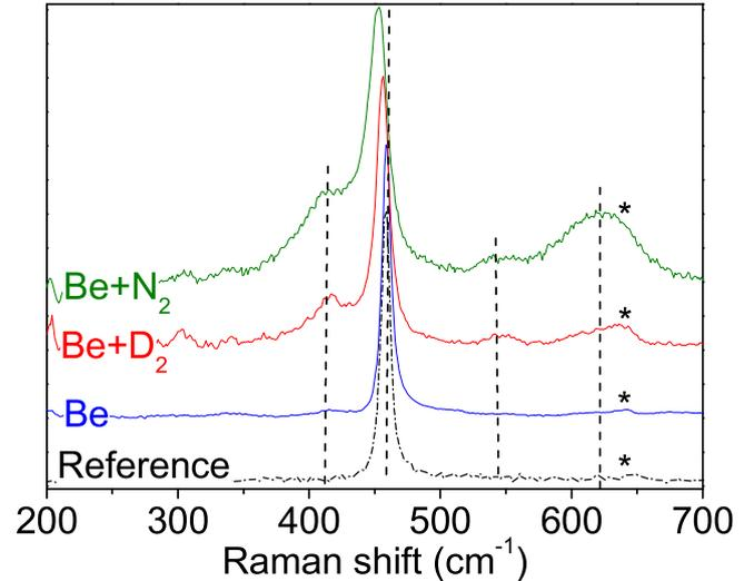
**Figure 1.** Normalized Raman spectra of Be, Be +  $\text{D}_2$  and Be +  $\text{N}_2$  samples. The dotted spectrum is Be polycrystalline sample. The star is one of the BeO bands according to [13].  $\lambda_L = 633$  nm.
