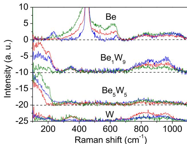
**Figure 2.** Raman spectra of the pristine Be, W,  $\text{Be}_1\text{W}_9$  and  $\text{Be}_5\text{W}_5$  samples deposited by TVA method. Color legends are the same as in figure 1.  $\lambda_L = 514$  nm.
