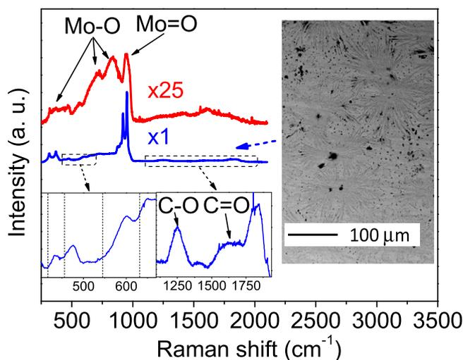
**Figure 3.** JET-92 mean Raman spectra corresponding to two zones on the sample. The upper spectrum is representative of the majority of the sample. The lower one is representative of a  $\approx 0.5 \times 0.5\text{ mm}^2$  region (right inset).  $\lambda_L = 325$  nm.
